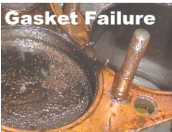
THE HEADGASKET WAS BLOWN BETWEEN CYLINDERS # 3 & 4.
